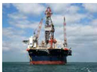
metres in height and the upper deck – 36.5 metres. The light weight is nearly 30,000 tons and the variable deck load is 15,000 tons. The rig is capable of working in water depth of up to 3,810 metres and has a drilling depth of 12,000 metres. The living quarters can accommodate 150 people and
